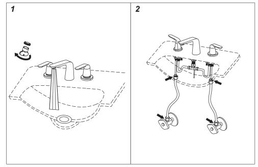
1. Remove the aerator by aerator wrench. Turn the faucet handle all the way on, turn on hot and cold water supply and flush water lines for one minute. Reinstall aerator by aerator wrench.
