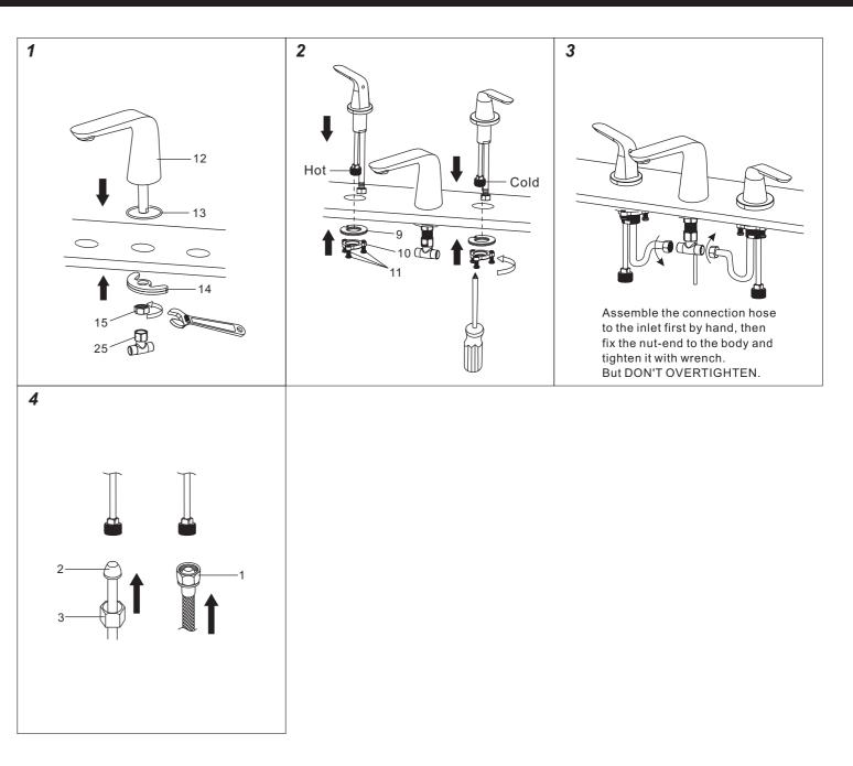
1. Position the o-ring #13 and body #12 in the installation surface as shown and secure it with gasket assembly #14 and tighten the lock nut #15 with adjustable wrench. Then assemble the connector assembly #25 to the faucet and tighten it with adjustable wrench. 2. Position the handle in installation surface as shown and secure it with fixing kit (#9,#11,#11) and tighten the screw #11 with screwdriver.
